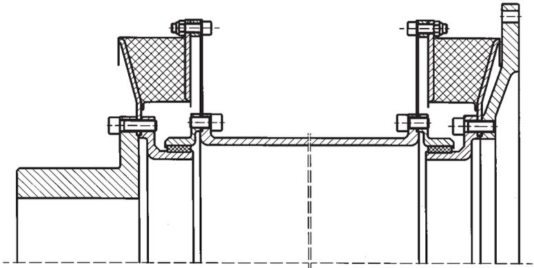
CENTADISC-flexible shaft, combined with torsionally soft CENTAX couplings in order to dampen torsional vibrations.
