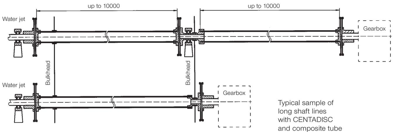
Typical sample of long shaft lines with CENTADISC and composite tube
