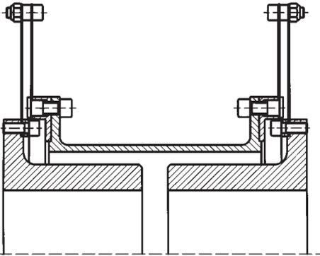
CENTADISC – short version with hubs inside the tube. Radial exchange not possible.
